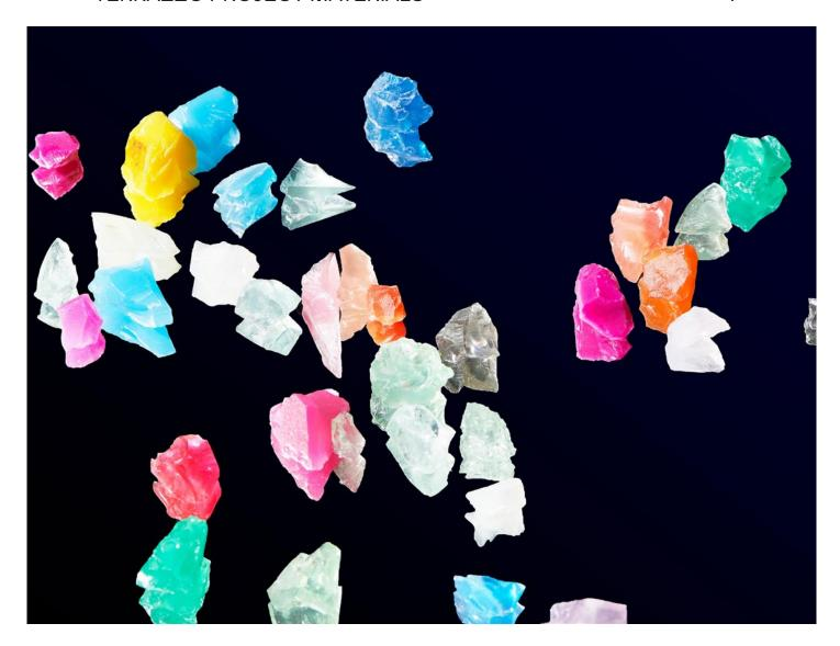
Terrazzo is a fascinating composite material produced from layers of cement interspersed by chips of stone — most commonly marble, glass or other appropriate aggregate. The mixture is sequentially poured, cured, sanded and polished until the desired finish is achieved. TP constantly develop new recipes using unexpected colour-ways and innovative material mixes to create crisp graphical surfaces.
